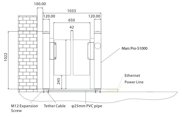
9. It is recommended that a warning line be marked on the ground after installing the device, so as to prompt the pedestrian to stand behind the warning line when verification.
