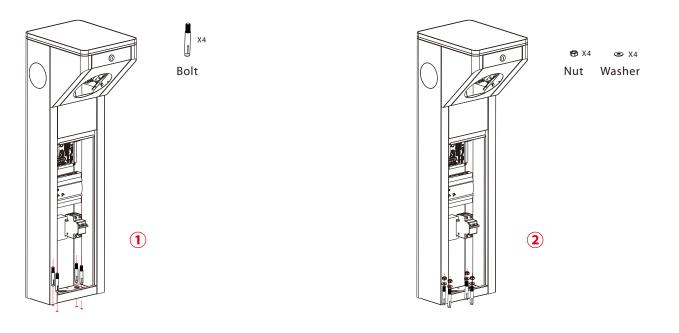
**Note:** Before inserting the bolt, the user must pull the power cable and Ethernet from the machines and put them into the wire slot.
