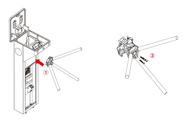
9. After assembling the arm, the resistance of the arm can be adjusted by rotating the damper left and right. Rotate the damper and observe the number on the damper. The greater the number it is, the larger the resistance will be.
